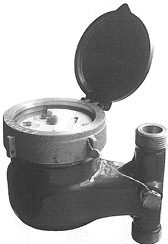
Figure 4: The water meter type MJ-LFC with plastic body – view and sealing:
